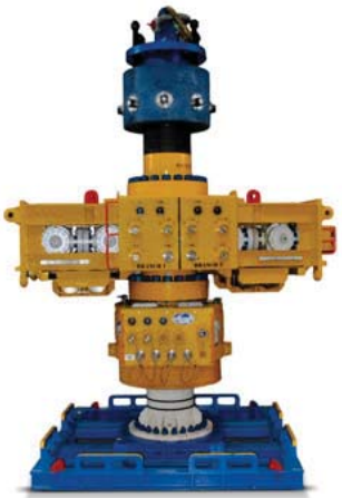
Figure 2: RWIS ready for mobilization, configured without shear rams
