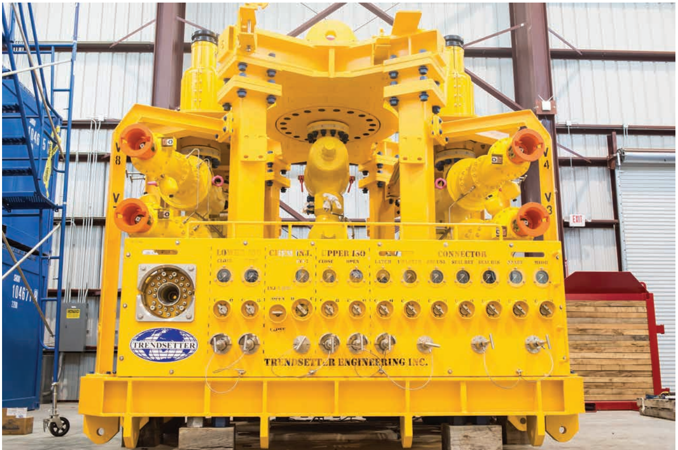
At the heart of this capping stack are two gate valves with a capacity up to 10,000 psi built for the Subsea Well Response Project's location in South Africa. Gate valves reduce the weight of the unit, which can be upgraded to 15,000 psi by substituting a higher-capacity blowout preventer in the otherwise standard design.
