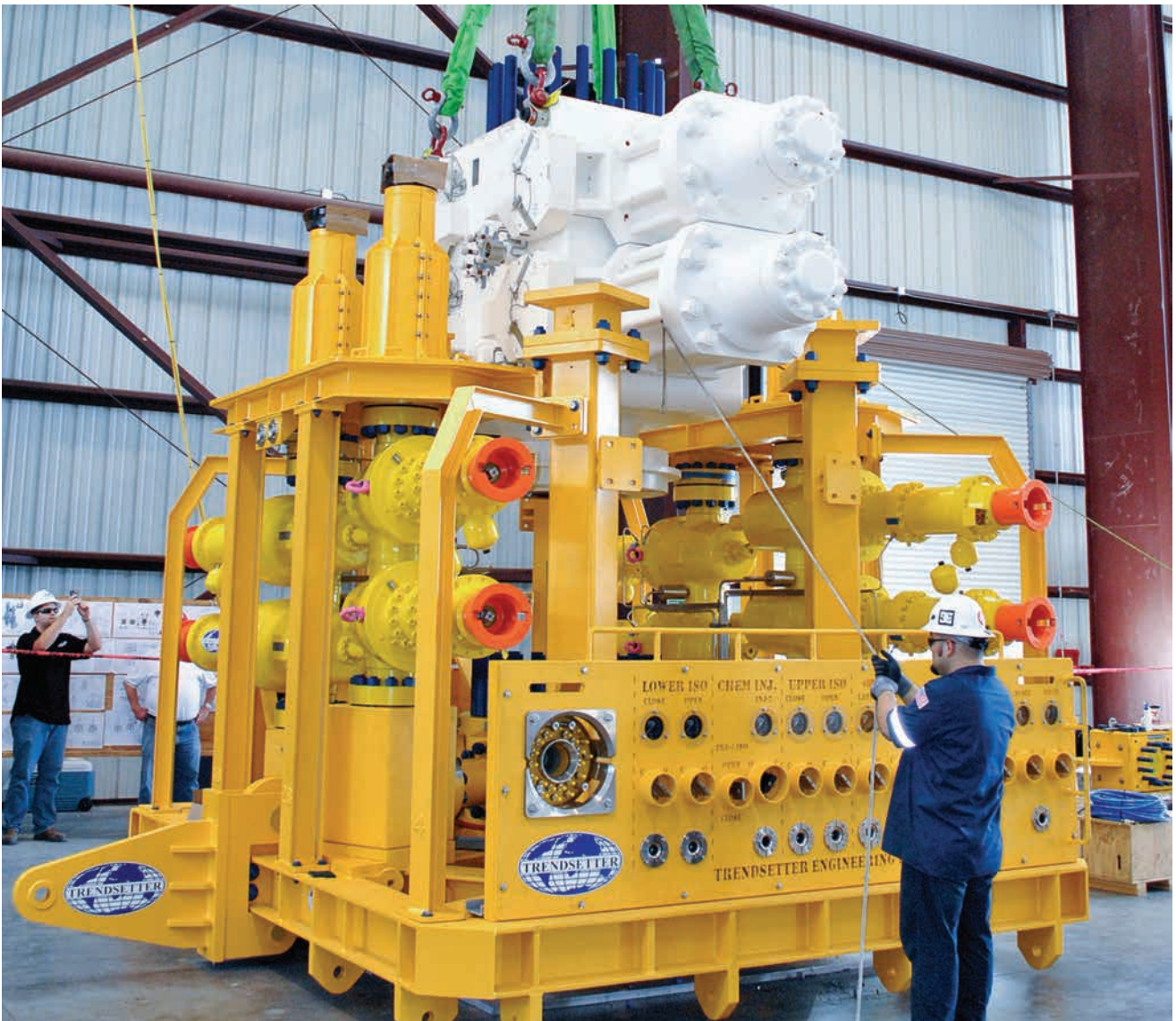
Workers lower a ram blowout preventer into a capping stack, giving it the power to shut down wells with pressures of up to 15,000 psi. If needed, this system built for the Subsea Well Response Project can produce up to 100,000 BOPD.
