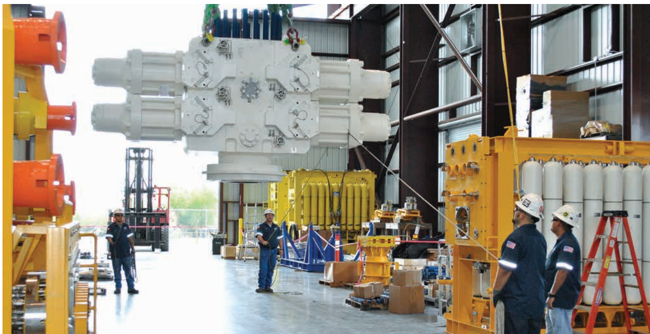
Workers lift a blowout preventer made by National Oilwell Varco that will be used in a capping stack designed to stand up to 15,000 psi.
