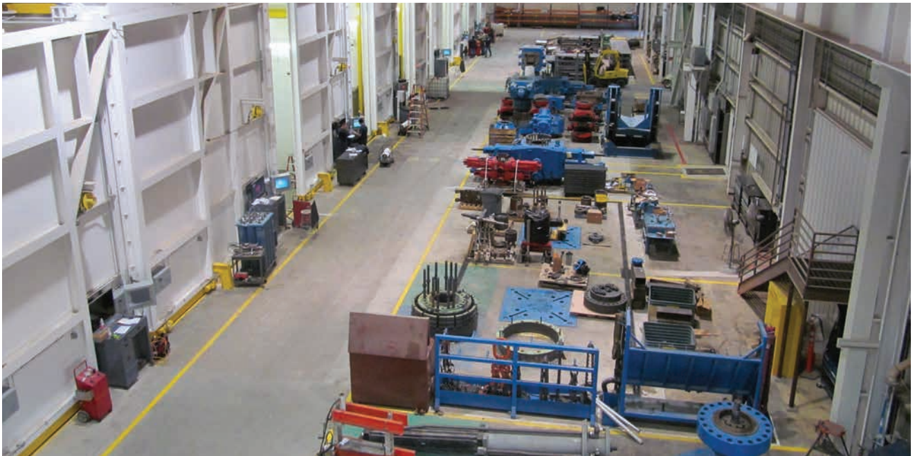
National Oilwell Varco's Pressure Control Group Research and Development Center was designed and is managed to increase the productivity of the work done there. To increase its productivity, test bays are organized in cells capable to performing a range of tests on multiple pieces of equipment, and on-deck areas nearby ensure equipment is set up and ready for testing when the next test bay is available.
