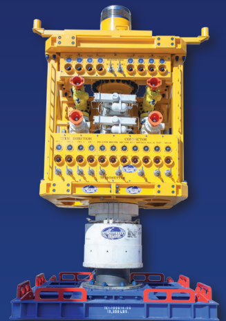
7 1/16" 10,000 PSI MWCC 10,000 FT WATER DEPTH 2X 4" OUTLETS
