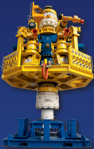
18 3/4" 15,000 PSI MWCC 10,000 FT WATER DEPTH 4X 5 1/8" OUTLETS
